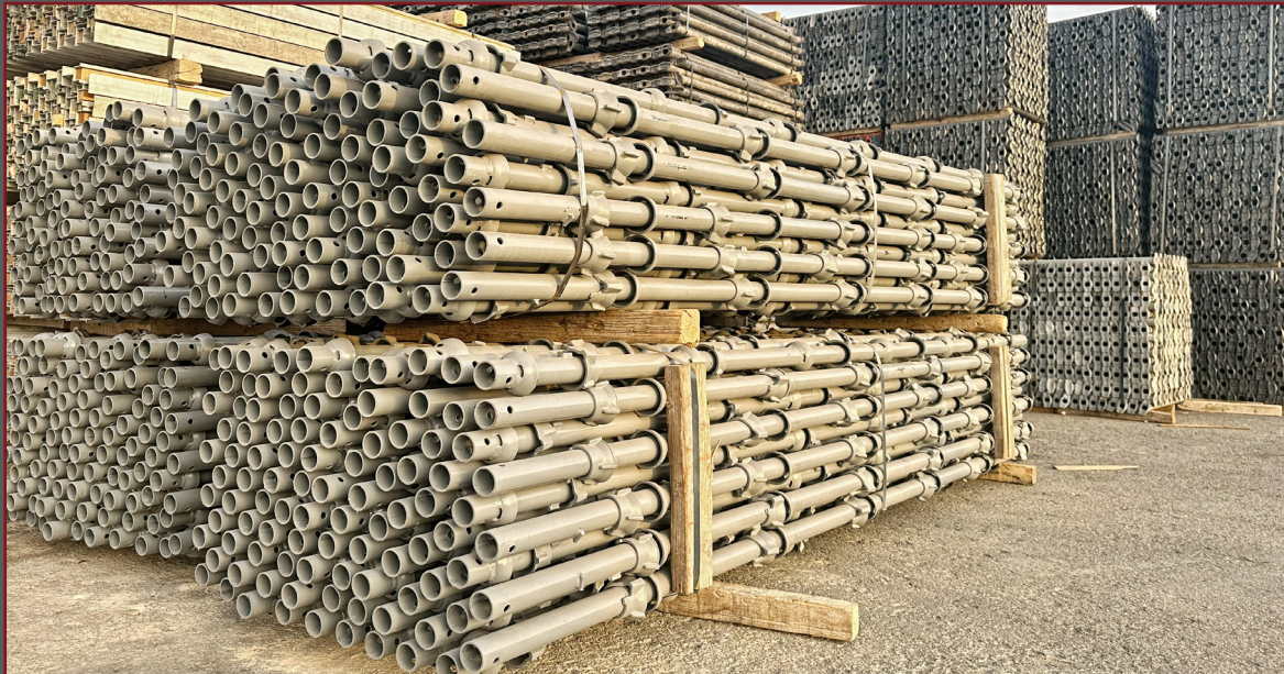
All S.felok Standards are manufactured from BS4360 grade 43 Embossed Tubes. Meet the requirement of EN 10219 of 320 N/mm' yield strength
