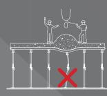
Overloading can cause the props to buckle and lead to the collapse of the shoring system.
